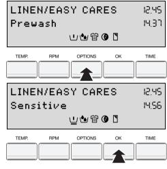
the option flashes and then press the OK key. The black bar under the symbol disappears.
